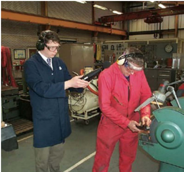
Making measurements with a hand-held sound level meter
